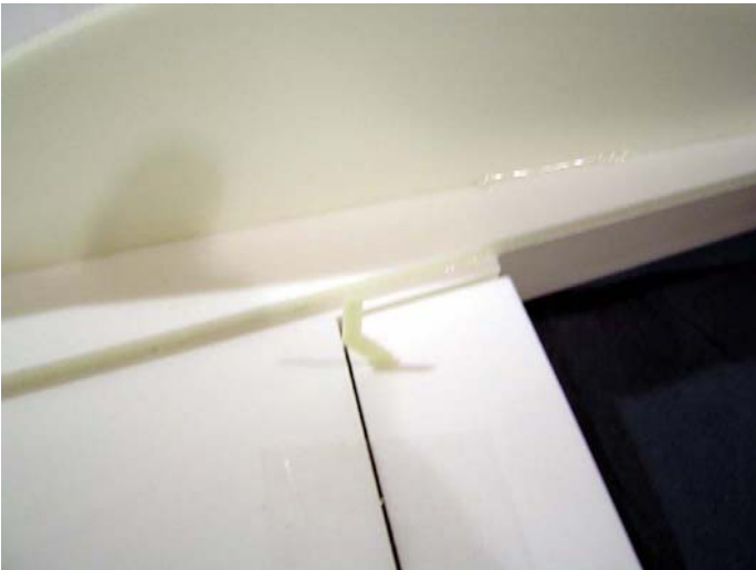
Install control hinges 1 inch on each aileron with arm on top of the wing.
