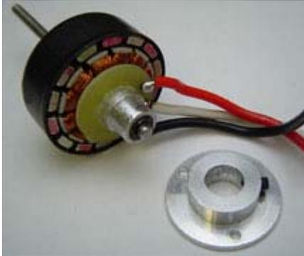
2. Pull off the firewall mount. Some twisting may be needed to get it all the way off.
