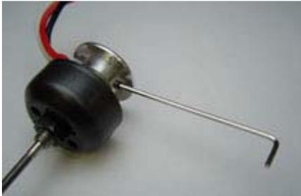
1. Use a 1.5mm Allen (hex) wrench to loosen the set screw holding the firewall mount on the back of the motor.
