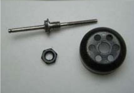
8. Remove the shaft from the bellhousing by tapping lightly on the front of the shaft. Always replace the shaft after removing it – you are sure to chew it up in the process of removing it. Reassemble the motor with the new shaft by reversing the disassembly steps.
