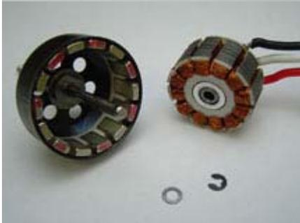
4. Pull the bell housing off the stator. The front bearing may come off with the shaft. If so, remove the bearing from the shaft and place it back in its boss on the stator. Since you have the motor disassembled, this is a good time to change the bearings also.
