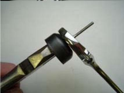
6. Take a deep breath, grasp the flange on the inside with the flat-nosed pliers and the nut with the crescent wrench and loosen the nut. It will be tight. Do your best to keep the jaws of the pliers tight up against the bellhousing to keep the pliers from slipping off the flange. We've found it is easier to hold the crescent wrench stationary, and turn the pliers like a screwdriver.
